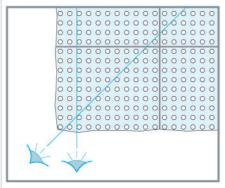
Check overall appearance of the ceiling constantly by alignment via the straights and diagonals of the perforation rows during installation (see drawings on page 4).
