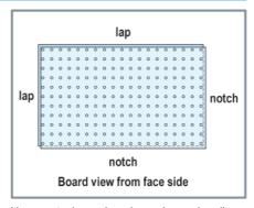
The special edge design of Cleaneo<sup>®</sup> Acoustic linear with one cut edge and one long edge each as linear notch and one cut edge and one long edge each as linear lap allow for an easy and precise alignment of apertura boards with continuous perforation. An installation team with 3 workers is recommended.
