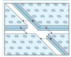
Always place linear notch edge adjacent to linear lap edge along front and long edges.
