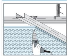
Fasten Cleaneo<sup>®</sup> Acoustic linear Boards with Drywall Screws SN 3.5 x 30 on metal grid made of CD 60x27 channels.
